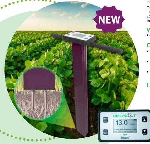
The TDR 250 offers the same proven time-domain measurement technology as the other TDR meters, but with a 20% less investment. The TDR 250 is a simplified portable soil-moisture meter that captures measurements in the root zone.
