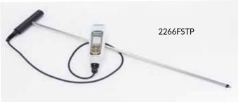
FieldScout Direct Soil EC Meter with 24 in (60 cm) T-Handle
